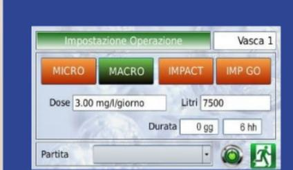
These two traditional functions are equipped, as per the innovative ones, with the control on the oxygen supplied, auto-compensation of both temperature and pressure, dose diagnostic, alarm on oxygen shortage and auto power off at the end of the treatment.
